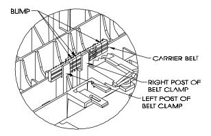
Figure 5-5. Carrier Belt Clamp.
